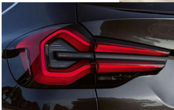
■ The **rear lights with full LED technology** make the rear view of the new BMW X3 seem even sharper. The distinctive, three-dimensional modelling of red areas with integrated turn indicators additionally underlines the presence of the rear end.
