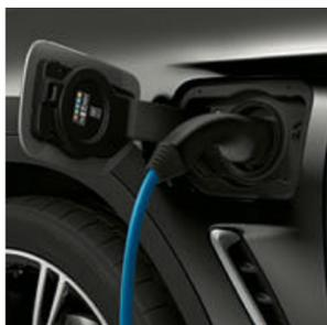
■ The charging socket of the plug-in hybrid technology including charging status display is concealed behind the charging flap in the front left fender.
